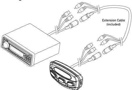
Once the remote has been mounted, connect the cables to the remote and head unit as in the diagram above. When routing the extension cable, be sure to avoid sharp objects, corners, and places where it might get pinched, as this could affect performance and cause damage to the unit.
